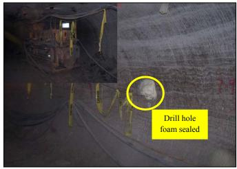
Figure 6. Virgin rock temperature experiment.
