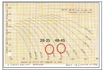
Figure 5. Main Fans Characteristics Curves.
