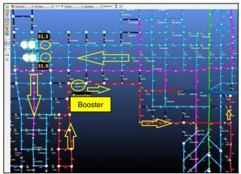
Figure 9. Scenario 1, Booster fan installation in Return.
