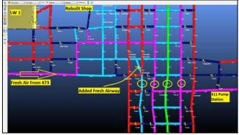
**Figure 13.** Scenario 5, Vetsim Visual Schematic View, Additional Fresh Airways.
