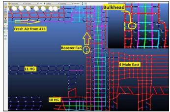
Figure 11. Scenario 3, The Location of Booster Fan in the Return Airway.
