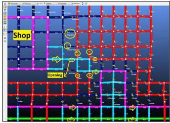
Figure 10. Scenario 2, Rerouting the Shop Air.
